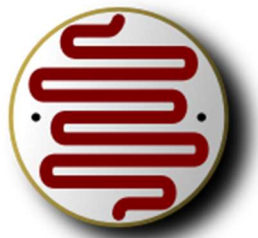
Light Dependent Resistor (LDR)
