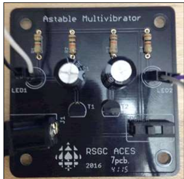
Astable Multivibrator Soldered PCB
