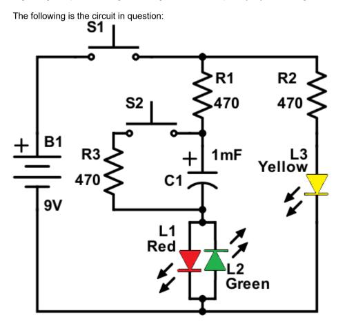
When S1 is closed, the circuit charges up C1 and illuminates the yellow LED. When the cap is sufficiently charged, S1 is opened and the user then closes S2. When in this configuration, both the green and yellow LEDs light up (and then dim as the capacitor voltage decreases). If the cap is fully charged and both switches are left open, the cap will gradually discharge through the green and yellow LEDs.
