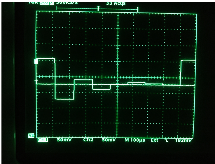
Fig. 5 Input signal (1.74V) and the DAC output signal of the SAR ADC
