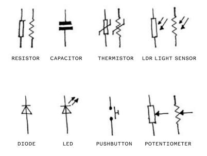
You may encounter variations in these symbols (for example, both variants of resistor symbols are shown here). See en.wikipedia.org/wiki/Electronic\_symbol for a larger list of electronics symbols. By convention, diagrams are drawn from left to right. For example, a radio would be drawn starting with the antenna on the left, following the path of the radio signal as it makes its way to the speaker (which is drawn on the right).
