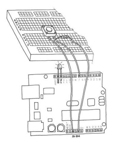
Figure 4-6. Hooking up a pushbutton
