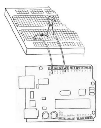
Figure 5-4. LED connected to PWM pin
