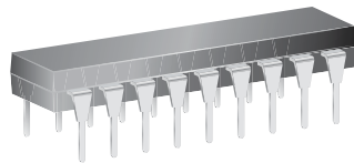
18-pin DIP (Package A)
